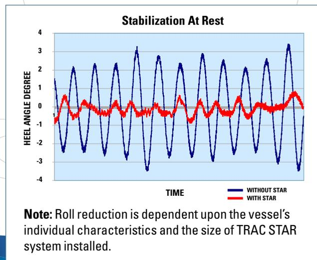
STAR (STabilization At Rest) is a system that significantly reduces vessel roll while anchored, on a mooring, or while drifting. STAR is a feature that can be added to most existing TRAC stabilizers and is available as an option on all new TRAC stabilizers.
